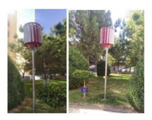
Vertical-axis wind turbines, as the name suggests, have the main rotor shaft positioned vertically. Unlike traditional horizontal-axis wind turbines (HAWTs) that have a horizontal rotor shaft, VAWTs have blades that rotate around a central vertical axis. This design allows them to capture wind from any direction and eliminates the need for a yaw mechanism to align with the wind.
